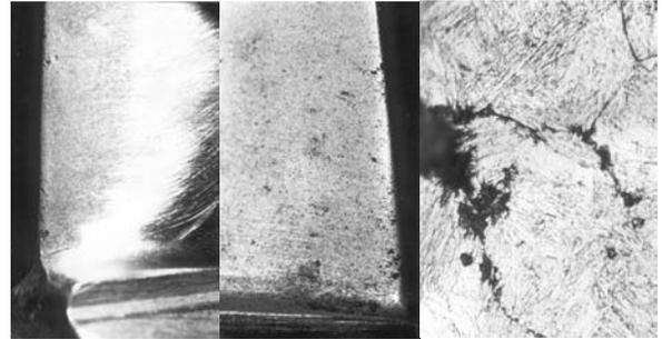
Fig. 14. Erosive-corrosive damage of the compressor blade made of martensitic steel following the operation [13].
