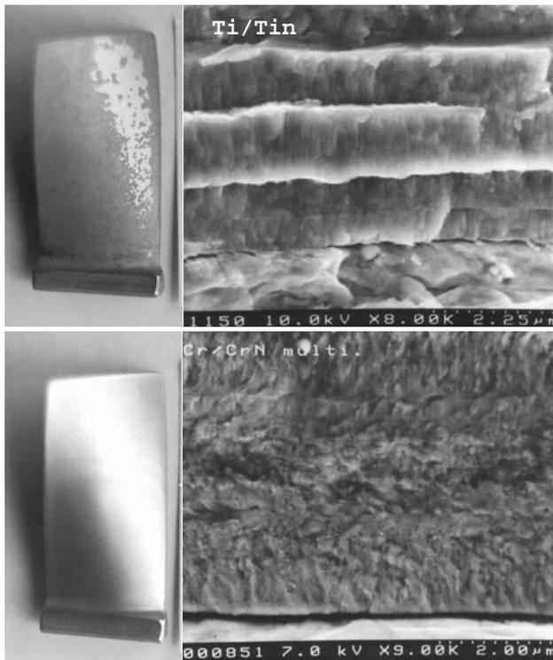
Fig. 16. Fracture morphology of Ti/TiN and Cr/CrN multilayer coatings deposited by Arc-PVD method on compressor blades made of martensitic stainless steel. View of coated compressor blades after engine test
