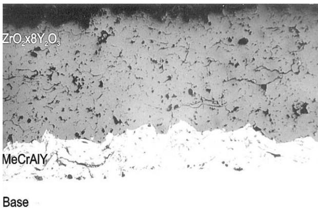
Fig. 9. The microstructure of plasma sprayed thermal barrier coating [L. Swadźba]
