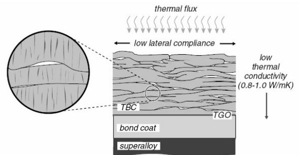
Fig. 11. The outline of thermal sprayed TBC microstructure [11]
