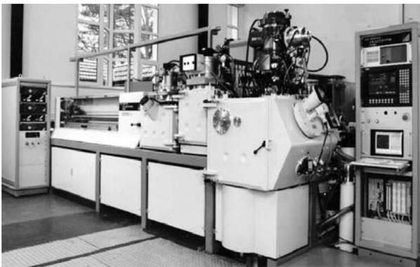
Fig. 13. The general view of EB-PVD TBC installation [12]
