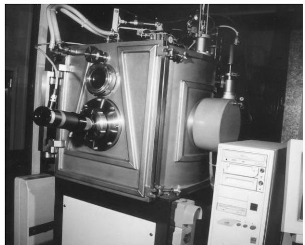
Fig. 15. The general view of the PVD equipment applied during the study on erosion and corrosion resistant coating deposition [B. Mendala]
