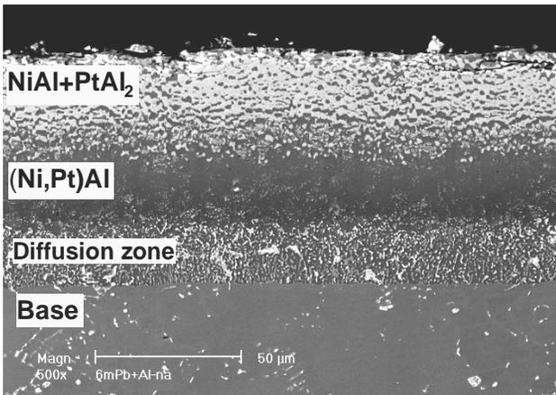
Fig. 6. The microstructure of platinum modified aluminide coating [8]
